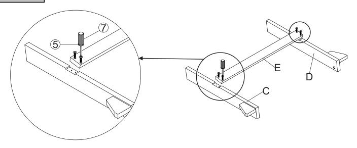
Attach Support Bar of Front Leg(E) to Left Front Leg(C) and Right Front Leg(D) using Screws(5) with Screwdriver(7).
