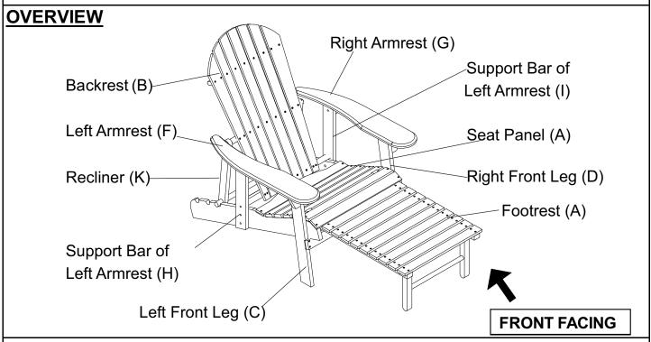
This Reclining Adirondack has multiple parts and may require up to 30 minutes to assemble. To give you an overview of the Reclining Adirondack parts, the above picture is to help you put the various parts into perspective. Please read through the instructions below to familiarise yourself with the parts and steps before assembly.
