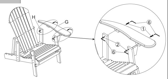
Attach Right Armrest(G) to Left Front Leg(C) and Support Bar of Left Armrest(H) using Bolts(1), and Sleeve Nuts(2) with Allen Keys(6).
