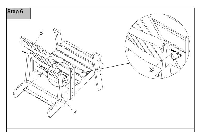
Position housing of Recliner(K) into oval mortise of Backrest(B). Secure Recliner(K) to Backrest(B) using Long Screws( $\Im$ ) with Allen Key( $\Im$ ) **Do not fully tighten the Screws**.
