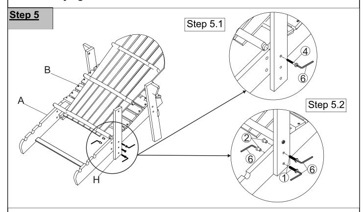
Place the Backrest(B) onto Seat Panel(A) as shown in the picture.
