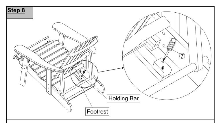
Reattach holding bars and screws from Step 2 to Footrest using Screwdriver(⑦). The holding bars are to prevent the Footrest from falling out of the Seat Panel. In a sequential manner, tighten all Bolts and Screws at all joints until fully locked into position.
