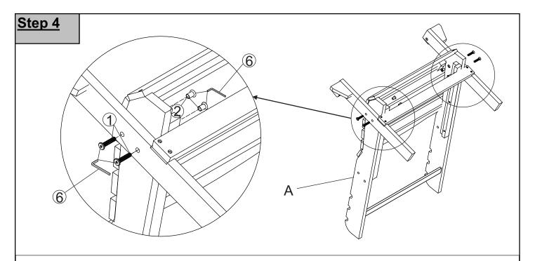
Stand the Seat Panel(A) vertically as shown in the picture. With the assistance of an adult helper, secure Front Leg Frame from Step 3 to Seat Panel(A) using Bolts(1), and Sleeve Nuts(2) with Allen Keys(6). **Do not fully tighten the Bolts.**
