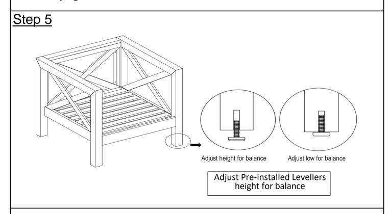
Inspect the Chair and make sure all parts are adequately connected. Carefully sit onto the Chair. This pressure will help align all parts at all joints. In a sequential manner, tighten all Bolts and Screws at all joints.
