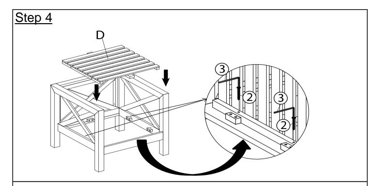
Attach Seat Panel(D) to the Chair using Screws((2)) and Allen Key((3)). Note: Insert Screws((2)) from inside to outside of Seat Panel(D). **Do not fully tighten the Screws.**
