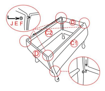
2. Secure table shelf (B) to table panels (C1,C2) by using 4 screws (E) and 4 washers (F) with allen wrench (J). Fully tighten all screws in step 1&2.
