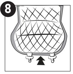
Finally, latch the hooks underneath your seat. WE SUGGEST WEARING PROTECTIVE EYEWEAR AND GLOVES FOR THIS STEP. You may have to look underneath or feel around for a secure place to hook your seat cover.
