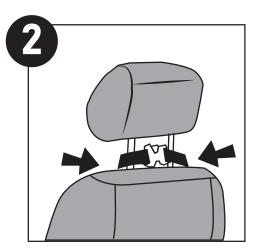
Attach the upper portion of the seat cover by connecting the buckle behind the headrest.
