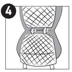
Lay the bottom portion of the seat cover onto the seat. Take the bottom cover's straps and loop each through a butterfly disc. Your seat cover should resemble the image above.
