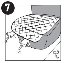
Optional: For a tighter fit, attach the hooks that are found in the bag to the bottom straps of the seat cover (you must pull open the hooks).
