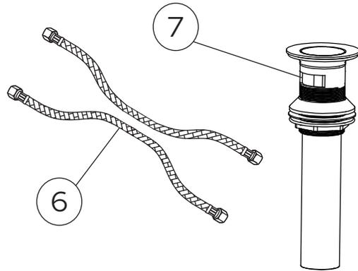
**!** Note: This faucet has been packaged with an over-flow pop-up drain. **DO NOT** use with a non-over-flow sink.
