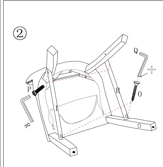
Caution: The bars H and I should be in horizontal position after installation. If not, the most possible reason is the rear feet were not installed correctly. Please check and swap the left and right rear feet.
