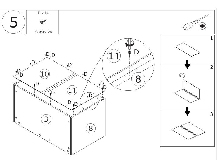
Fix back board 10 and 11 to the component with screw(D) as shown.
