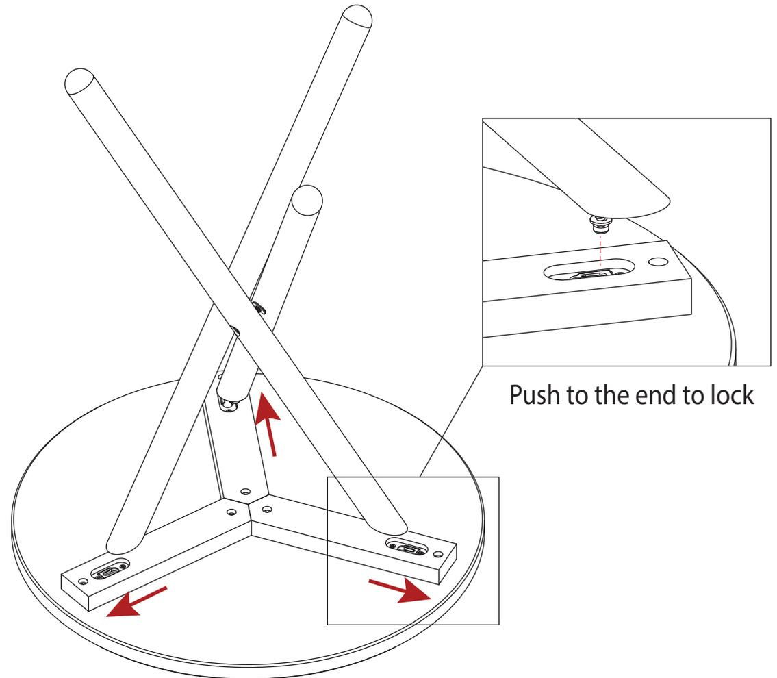
Put the first leg in the hole and push it to the end, with the other two legs to the hole at the same time and slide to the end to lock.
