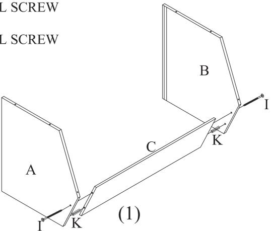
For PART C, be sure the correct side without visible hardware is facing out. For PART E (in Step 2), the side with the countersunk holes faces out.
