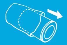
Remove outer plastic bag from PRO-Cell filter.
