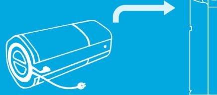
Plug power cord into Skye and wrap any excess cord around the base.
