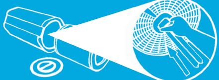
Hold the base of the lamp and plug into Skye until you hear a click.
