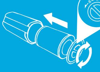
Place the "PRO-Cell" filter back into Skye. Close the base cover by aligning the arrows and then turning clockwise into the locked position. If the cover is not completely flush with the base, the unit will not operate.
