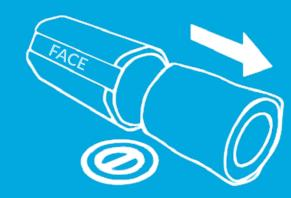
2 Remove the PRO-Cell filter from Skye.
