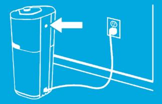
Plug the power cord into a power outlet and tap the power button (on back).
