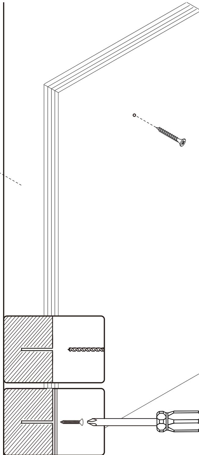
**EN** If it is a solid wall, please use expansion and self-tapping screws, if it is a wooden wall, only use self-tapping screws, please do not overtighten the screws
