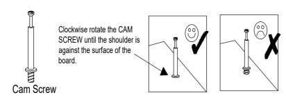
Insert the CAM SCREW into the HIDDEN CAM. Clockwise rotate to tighten the HIDDEN CAM.
