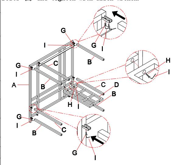
STEP:2. Repeat Step#1 to connect another Metal frame (A) with the assemblied unit as diagram shown.
