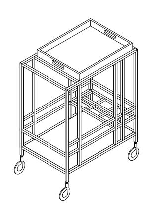
STEP:3. Lay down the assemblied unit on a clean and soft surface, then insert the Wheel(J) into the bottom of legs as diagram shown, and tighten them with wrench (L).
