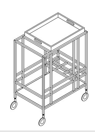
STEP:1. Connect metal frame (A) with metal tubes (B/C) through Bolts (G) as diagram shown and tighten them with allen wrench, then connect the metal shelf (D) onto the assemblied part with Bolts (H) and tighten with allen wrench.
