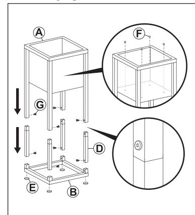
Apply four Protective Feet (E) to the bottom of Base (B).
