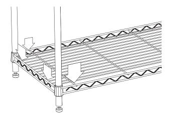
Snap half-sleeve sets onto all four posts at the desired height for the NEXT shelf. Lower this shelf into position and press until fully seated. Install the third and fourth shelves in the same manner, with both shelves mounted ABOVE the post seams.
