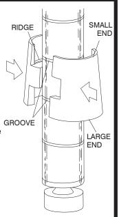
Stand a D Shelf on end, and from the BOTTOM side of the shelf (the bottom side is recessed), slide the TOP end of a post through a corner hole until the half-sleeves are seated in the corner hole. Repeat with remaining posts.
