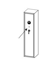
NOTICE: Use the emergency key when opening the door for the first time. After installing the battery, set the fingerprint password and key password
