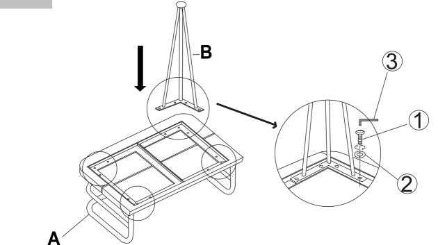
Insert leg (B) into the seat panel (A), put the flat washers (2) and bolt (1) as above picture.
