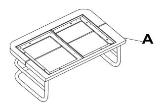
Lay the Seat panel (A) facedown onto a clean, flat surface to avoid any scratches or damage to the product.
