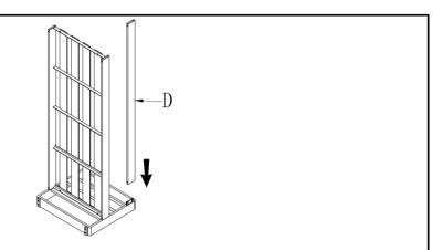
Insert the Back Support Bar(D) into the Left Side Panel(A).
