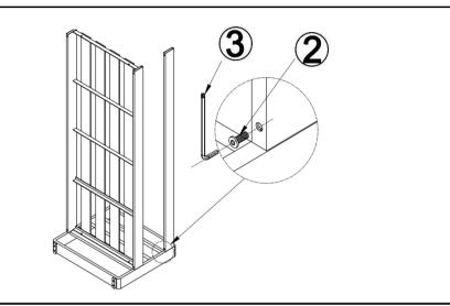
Attach Back Support Bar(D) to the Side Panel(A) using Bolt(②) with Allen Key(③). **Do not fully tighten the Bolt.**
