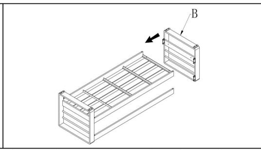
Insert the Right Side Panel(B) into the Back Support Bar(D) and Seat Panel(C) as shown above.
