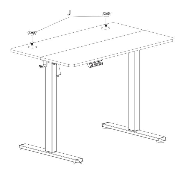
Insert Cable Hole Cover J\*2 into the hole in the Board 9a.
