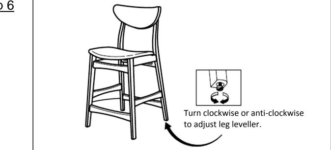
Turn clockwise or anti-clockwise to adjust leg leveller. The **Max** height during 0.25~0.8inch.
