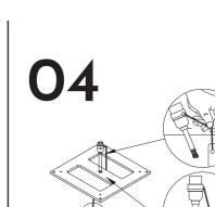
Grab your lampholder board (I) and ensure that the pull chain falls into the open hole then tighten the lampholder using the screw on the wire.
