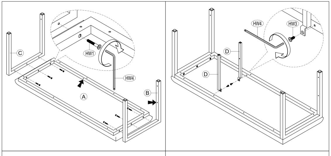
STEP 1 ATTACH LEG FRAMES 1 AND 2 (B AND C) TO CUSHION (A) USING BOLTS 40 MM (HW1). TURN BOLTS USING ALLEN KEY (HW4); NOTE: ATTACH BOLTS ONLY HALFWAY THIS TIME.
