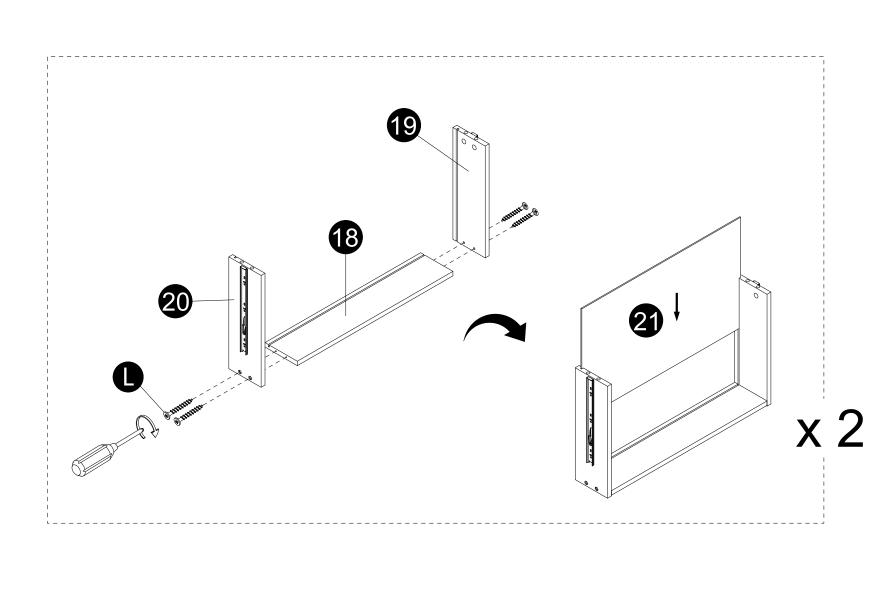
$\cdot$  Attach panels (19,20) to panels (18) with screws (L) correctly.
