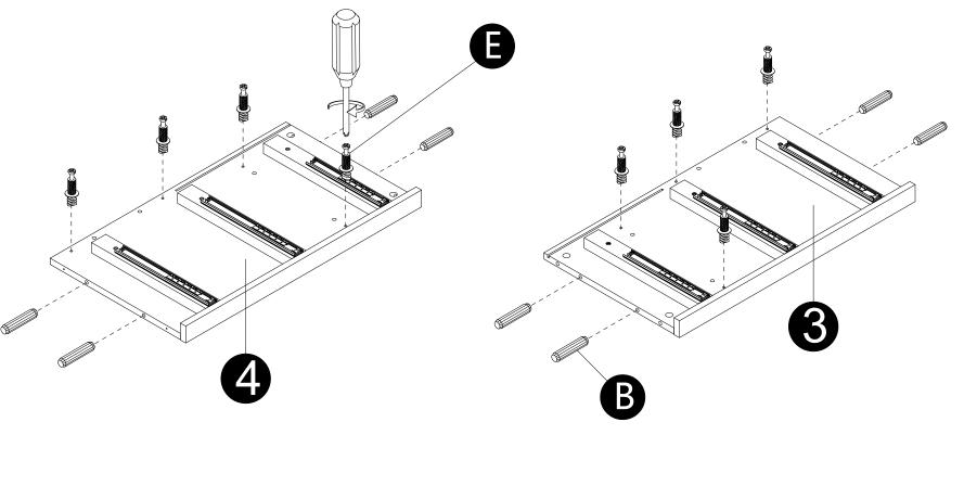
Screw cam bolts (E) into panels (3,4).
