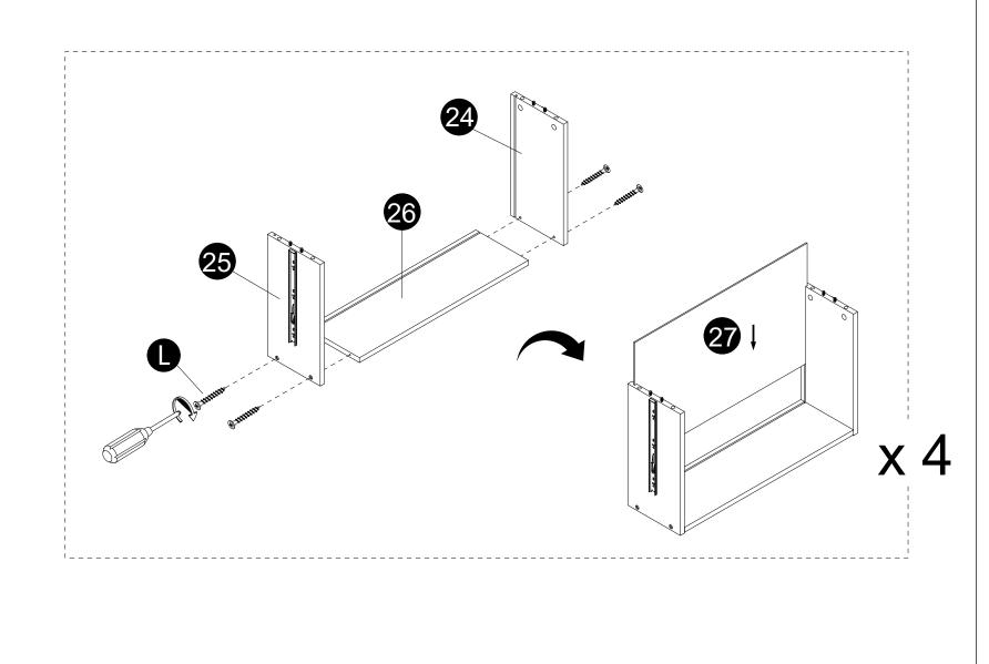
$\cdot$  Attach panels (24,25) to panels (26) with screws (L) correctly.
