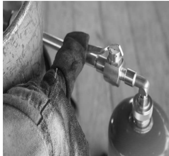
Depressing Dead Man Valve to fill 1 lb. Cylinder
