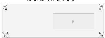
b. Use the proper anchorage hardware such as screws and washers (depending on the material of the surface you are anchoring the unit to). Anchor the unit via the 4 screw holes 'A' found at the base of the unit. Access the anchoring holes through the burner slot 'B'.
