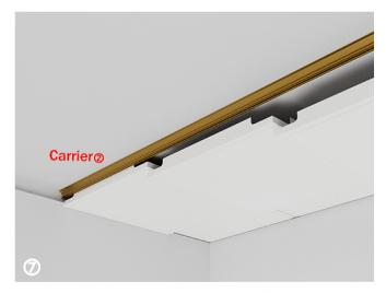
The two edge of the ceiling panel are respectively clip into the carrier  $\hat{\mathbb{Q}}$  and carrier  $\hat{\mathbb{Q}}$ .
