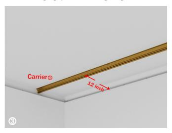
Then, install the carrier  $\hat{\mathbb{1}}$  on the top with screws, and the center of the carrier is 12 inch away from the wall.
