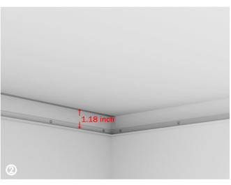
First, use screw or sealant to install the L angle on the surrounding walls at the place 1.18 inch away from the roof.
