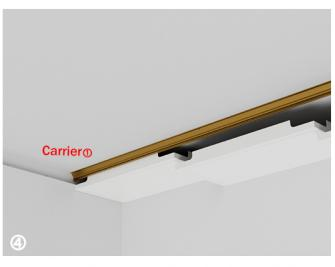
Place one edge of the ceiling panel on the L angle,  $\,$  and clip the other edge into the carrier @
