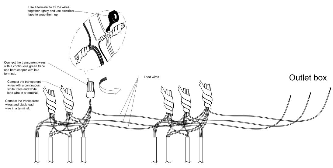
Remark: Every terminal can fix maximum 5 wires, if there are more than 4 fixture wires to be combined, please use more terminals to connect the wires.
