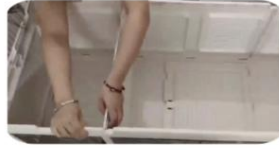
2. Unfold the surrounding panels and align them with the snap fasteners to secure them
