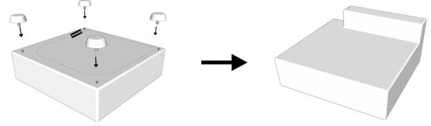
4. Insert the 4 latches into the built-in buckles of the armrest and backrest respectively, and install the armrest to the low position and the backrest to the high position through the latches.
