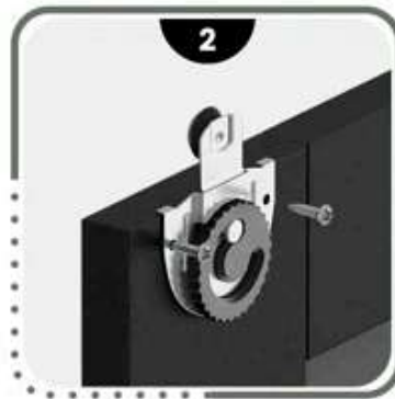
Attach the roller to the door
