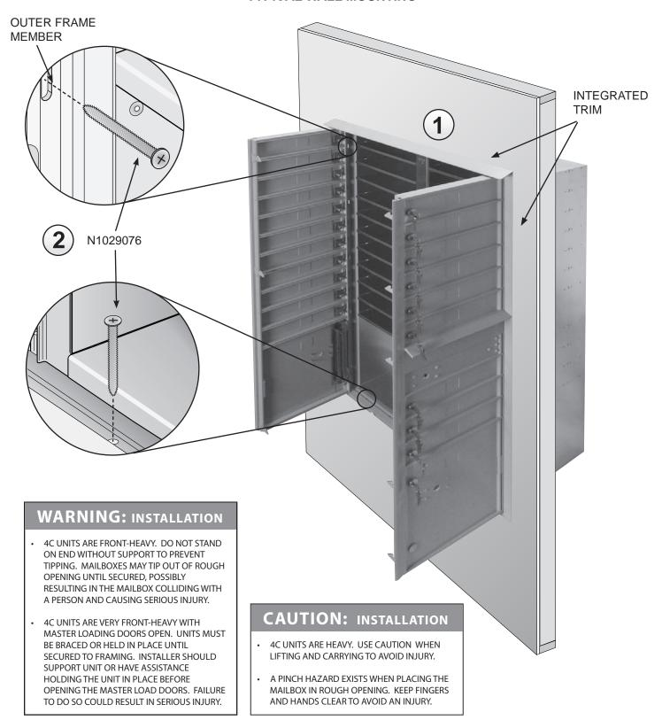
NOTE: N1029076 #8x2" LONG WOOD SCREWS SHOULD BE TIGHTENED TO ENSURE A SNUG FIT. HOWEVER, OVER TIGHTENING BEYOND INITIAL CONTACT WITH FRAME COULD HINDER FUNCTIONALITY. IF OVER TIGHTENING OCCURS, SIMPLY BACK OUT EACH OVER TIGHTENED MOUNTING SCREW.
