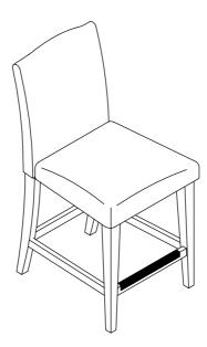
ADDITIONAL NOTE ABOUT SAFETY: BOLTS MAY LOOSEN DURING NORMAL EVERYDAY USE. THEY SHOULD BE PERIODICALLY INSPECTED AND RE-TIGHTENED TO PREVENT DAMAGE OR INJURY. ALWAYS CHECK TO ENSURE THAT ALL HARDWARE IS KEPT TIGHTENED.
