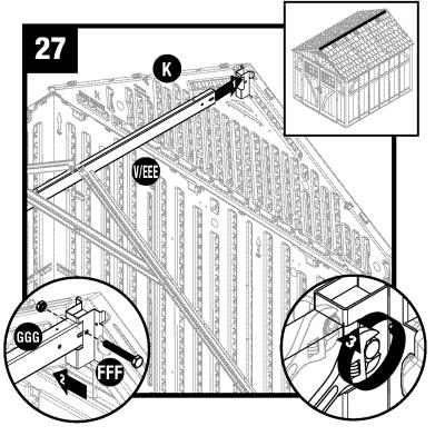
Raise ridge beam (V/EEE) up and into rear header (K). Secure with one bolt (FFF) and one nut (GGG). DO NOT tighten. Repeat for front header (J).
