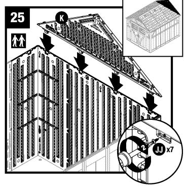
Place rear header (K) over back walls and fit four protruding support legs into pockets molded in back walls. Secure rear header using seven screws (JJ).
