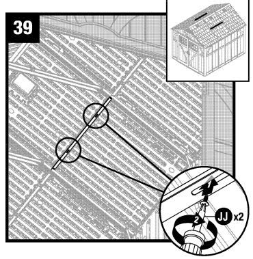
Secure roof support extension (BB) to inner roof panel using two screws (JJ).
