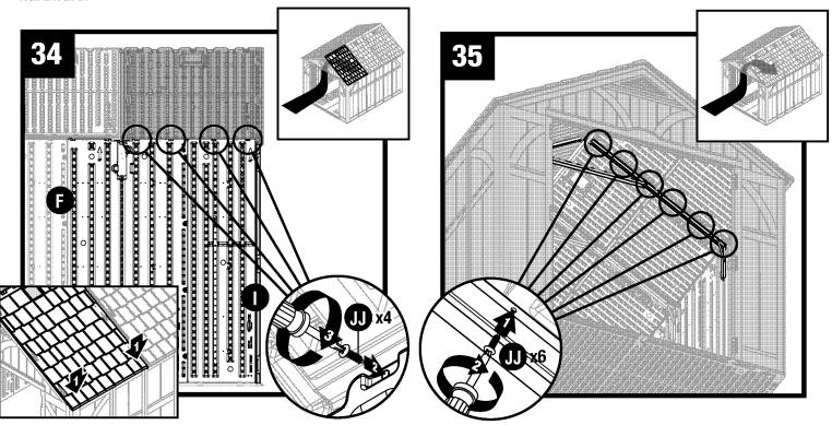
Pull down each lower corner of roof from outside. From inside shed, attach tabs on right front corner (I) and side panel (F) to roof panel with four screws (JJ).
