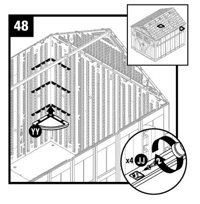
Attach shelf (YY) in desired location with four screws (JJ) Repeat for remaining shelf (YY).
