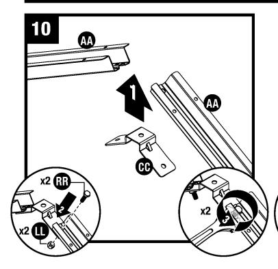
Attach truss bracket (CC) to end of one truss leg (AA) with one hex bolt (RR) and one nut (LL).
