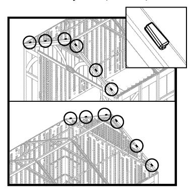
Before proceeding, locate and identify six front header tabs and six rear header tabs.
