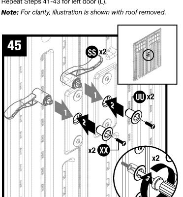
From the outside of doors, insert door handles (SS) through handle plate holes. On inside of doors, place spacers (UU) on each door handle, and secure each with one machine screw (XX).
