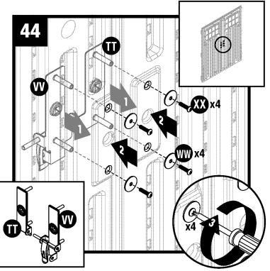
Insert screw stems, on left and right handle plates (TT) and (VV), through the pre-drilled holes in doors. While holding plates in place on exterior of door, secure each with two washers (WW) and two machine screws (XX).
