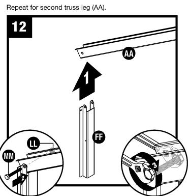
Attach side adaptor bracket (FF) at end of left truss leg (AA) with one cap screw (MM) and one nut (LL). Repeat for remaining side adaptor bracket (FF).
