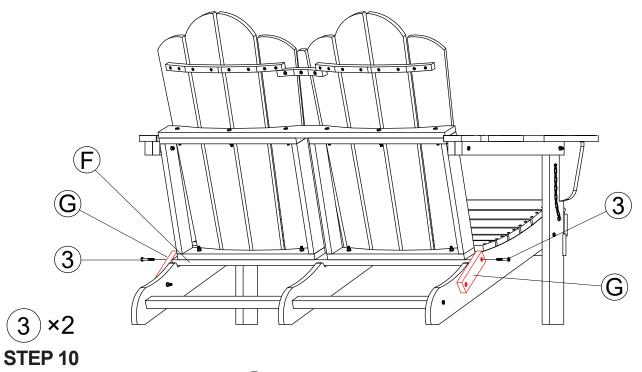
As shown in the figure, use 3 to fix G and F.
