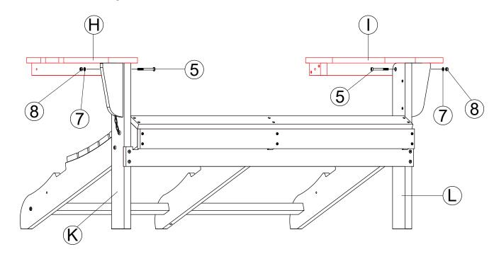
(5) ×2 (7) ×2 (8) ×2 STFP 7 As shown in the figure, use 578 to fix H, I and K, L
