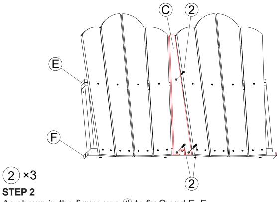
As shown in the figure, use (2) to fix C and E, F
