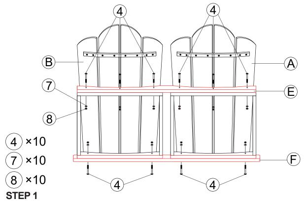
As shown in the figure, use (4)7)(8) to fix A, B and E, F
