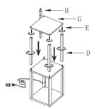
2.Screw three poles (D) into the exposed part of the two-side bolts (E). Take the LED pole with the direct current connector (H) and connect it with the exposed part of the direct current connector. Then, screw the two-side bolts (E) into the three poles (D) and place the middle board (G) on the bolts.
