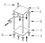
1. Assemble the lamp base by screwing bolt(B) three poles (D) and an LED pole with wire (F) clockwise into the thick baseboard (C) until tight. Place the cushion (A) to cover each hole. Then screw the two-side bolts (E) into three poles (D) and place the middle board (G) on the bolts. Ensure that the big hole on the board is on the same side as the LED pole with wire (F).
