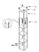
4.Screw four poles (K) into the exposed part of the two-side bolts (E). Ensure that the installation groove of the light shield on the pole (K) faces inwards. Insert the four light shields (L) into the installation groove of the light shield. Then, tighten the bolts (B) clockwise to secure the top board (M) and the four poles (K) until they lock.
