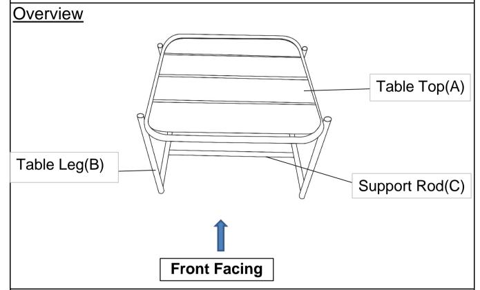
This Table has multiple parts and may require up to 20 minutes to assemble. To give you an overview of the Table parts, the above picture is provided to help put the various parts into perspective. Please read through the instructions below to familiarise yourself with the parts and steps before assembly.
