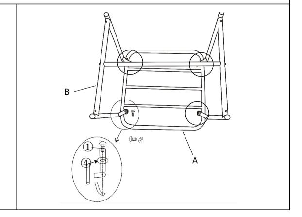
Attach Table Leg (B) to Table Top (A) with Bolts(1) and Washers (4) using the Allen Key (3).
