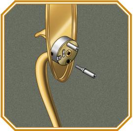
**6** Screw the lower post into the threaded hole at the bottom of the thumblift cartridge and tighten.
