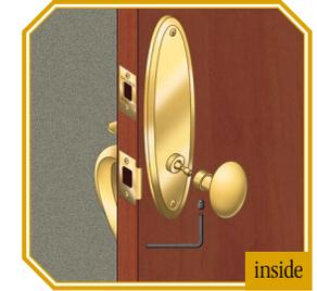
**5** Slide knob/lever onto dummy inside adapter and tighten set screw with Allen wrench. Position knob/lever with set screw down and toward hinges. Knob/lever is secured when set screw enters V groove in spindle.
