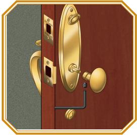
**1** Loosen the set screw using the Allen wrench provided. Remove the knob or lever from the spindle.
