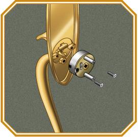
**1** Remove the #6-32 x 7/16" flat head screws that secure the thumblift cartridge to the handleset. Discard the cartridge and the screws.
