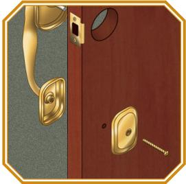
**6b** Supporting the handleset with one hand, unscrew and remove the lower #10-32 x 2 1/4" oval head screw and screw cover backplate. Remove the handleset.
