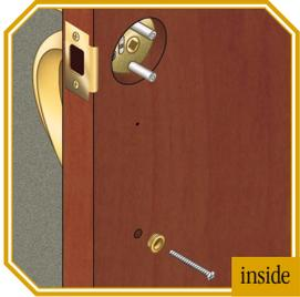
**1a** Attach bottom of outside handleset by inserting the #10-32 x 2½" flat head screw on inside of door through screw cover backplate, lower hole, and into outside handleset. Leave screw loose for later adjustment.
