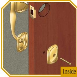
**1b** Attach handle by inserting the #10-32 x 2¾" oval head screw on inside of door through screw base and the lower hole. Leave screw loose for adjustment.
