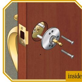
**2** Place the new dummy inside adapter on the door, aligning the holes in adapter with posts on outside handleset. Secure with two new #10-32 x 1¼" truss head screws.
