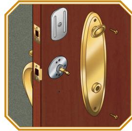
**3** Remove the screws securing the interior escutcheon plate and remove escutcheon plate. Put the escutcheon and screws to the side for reassembly later in the installation.
