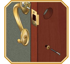
**6a** Supporting the handleset with one hand, unscrew and remove the lower #10-32 x 2 1/2" flat head screw and screw cover backplate. Remove the handleset.
