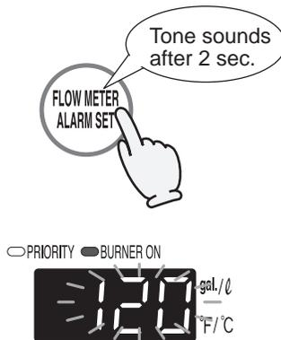
**3** Change the temperature using the setting buttons.
