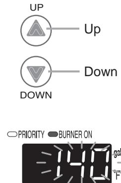
The upper limit of the hot-water supply temperature can be changed to
