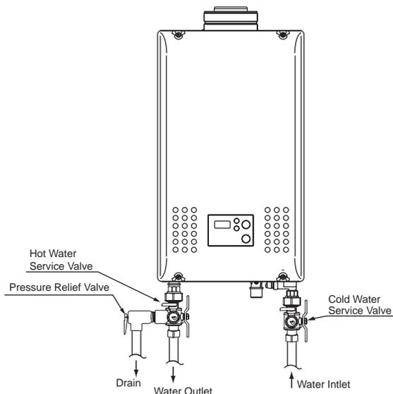
\* Isolation valves may be purchased as an accessory from Noritz. They allow for full diagnostic testing and easy flushing of the system.
