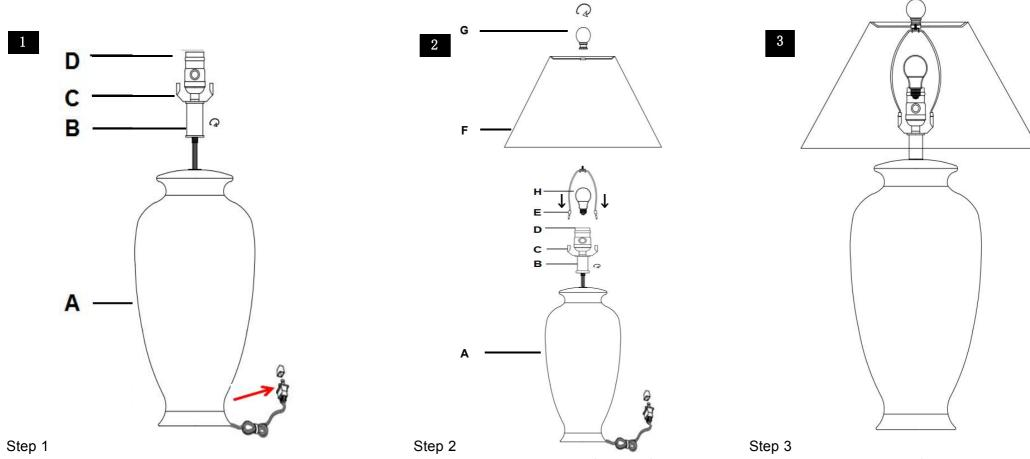
Pull power cord to connect the Neck (B) to the Base (A). Screw the Neck (B) onto the Lamp base (A) Be careful not to twist the power cord and tighten securely Insert the Harp (E) into the Saddle (C). Put the shade(F) on the Harp(E), then tighten the Finial (G)into the Harp (E) Insert the bulb(H) into the socket(D). Step 3 Put the light on a level surface to check if everything is stable.
