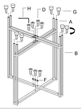
Attach assembled metal base to Wood Top (C) by Bolt (E) and Allen Wrench (H) as shown.
