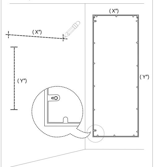
■ Measure the distance between the mirror hooks and measure the same size on the wall.
