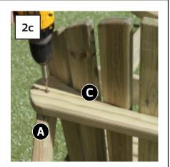
Locate Back Assembly C as shown in Fig 2a and fix in position using 6no Screws. (Figs. 2b & 2c).
