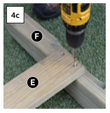
Ensuring correct orientation of Rockers F (larger cut-out to rear and innermost), position Rocker Brace E onto front of Rockers F (Fig.4a & 4b) and secure in position using 4no Screws (Fig.4c).
