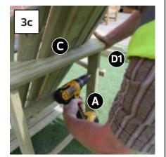
Position Armrest/Leg Assembly D1 as shown in Fig.3a. Align bolt holes and insert 2no Hex Bolts and 'T' Nuts. (Fig. 3b). Do not fully tighten.
