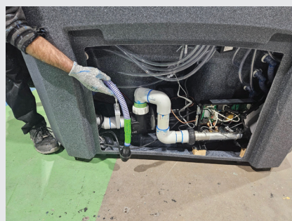
FIGURE 1.4C -- DRAIN VALVE ON ARISE SPA
