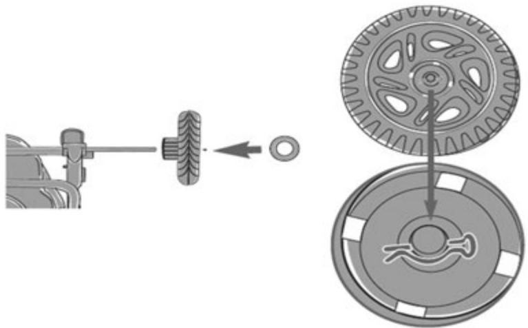
**Step 4.** Line up each of the tabs in the hub cap with the slots in the wheel, snap hub cap into place.
