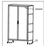
Install casters: Screw the casters into the threaded pipe race at the bottom of the side frame. Attention: During installation, support the cabinet to prevent tipping. Finally, remove the protective film from the cabinet door to complete the installation.
