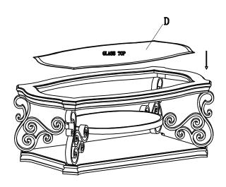
STEP 4: Turn over the table. Tighten all bolts carefully and Insert Glass top (D) into the Top Frame (A)
