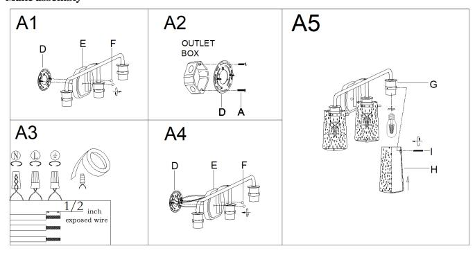
Step A1: Unscrew the studs(F) from the back plate(E) then gently remove the mounting plate (D).
