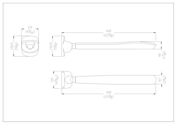
These ergonomic design folding rails are an important feature for persons requiring some support in either the shower or toilet. Manufactured from warm to touch PE-LD material and strengthened with a steel tube running through the core. The fixing plate is made from stainless steel and has a special plastic gasket which prevents damage to the wall or tiles. Inside the
