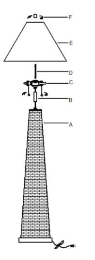
1.Fasten The Lamp body A Into The Base. Becareful not to Twist The Power Cord.
