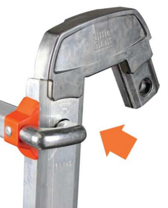
Engage the lock tab completely into the trestle bracket.
