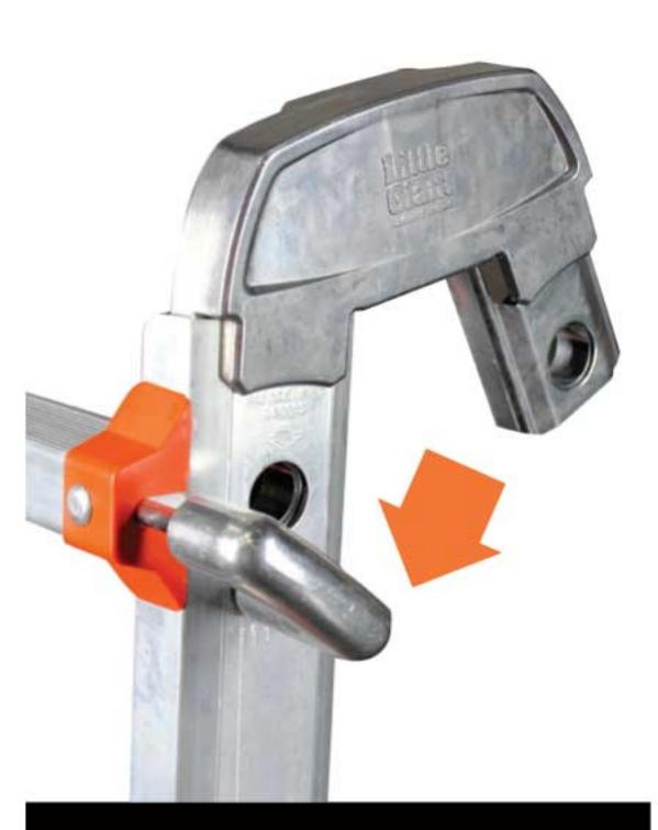
Unlock the lock tabs. Insert the trestle bracket with the flange on the outside of the rail.
